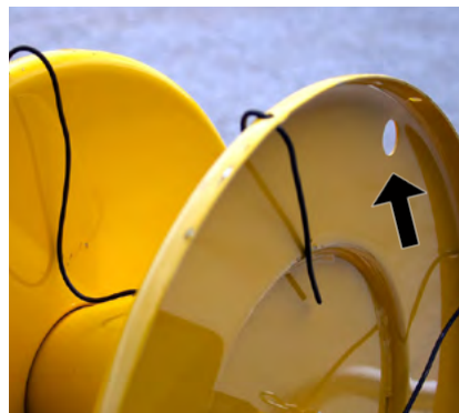
Wire tie off for wire being rolled
