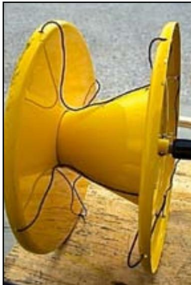
8) There will be (4) holes in the outside edge of the reels. These are to mount tie wires, before you start rolling wire. You will use the same system for standard reels(as shown), as well as Magnum reels. (We used #9 wire for the picture, but regular electric fence wire will work fine)
