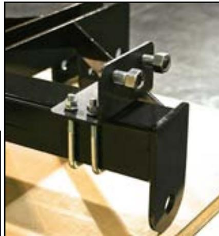
2) Mount the magnum carrier arm bracket to the opposite end of the tool bar. Leave this loose until the whole unit is assembled, there will be adjustments as you assemble the unit.
