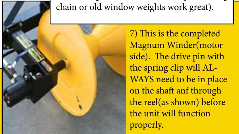
7) This is the completed Magnum Winder(motor side). The drive pin with the spring clip will ALWAYS need to be in place on the shaft and through the reel(as shown) before the unit will function properly.
