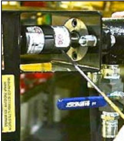
6) Once everything is aligned, tighten the (2) 1/2" bolts that hold the motor in place. Also, tighten the set-screws on both Lovejoy coupler halves.
