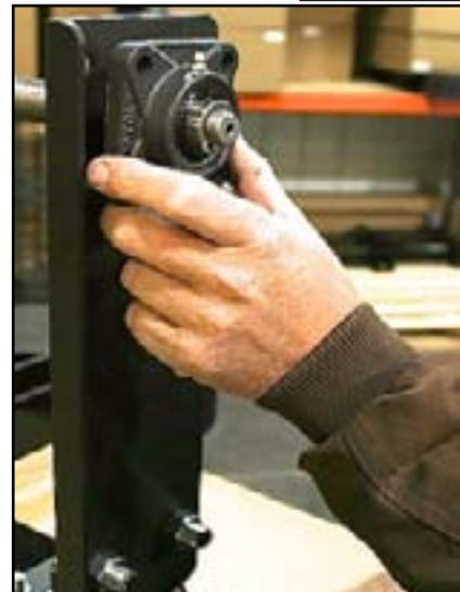
3) Set the carrier bearing plate in place(as shown), mount the bearing with the (4) 5/16" bolts provided. Then, using (2) 5/8" nuts, you can bolt the bearing plate in place with the angle bracket that comes off the tool bar. ALWAYS have the 3/4" nut in place on the end of the shaft before rolling wire.
