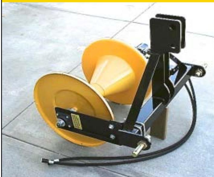
\*\*\*When unrolling wire, tie the wire to corner post and put hydraulics in float position. At this time of operation, have the ball valve fully opened. This allows oil to circulate through the hydraulic motor, acting as a drag to help avoid aggressive unspooling. If you need to stop, the circulating oil will stop the reel from turning.
