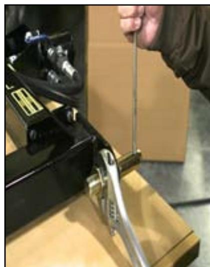
4) Install the pins on the draw bar mount of the winder. Category 2 & 3 pins will be 1/18" and mounted outward(as shown). Category 1 pins will be 7/8" and mounted towards the inside.
